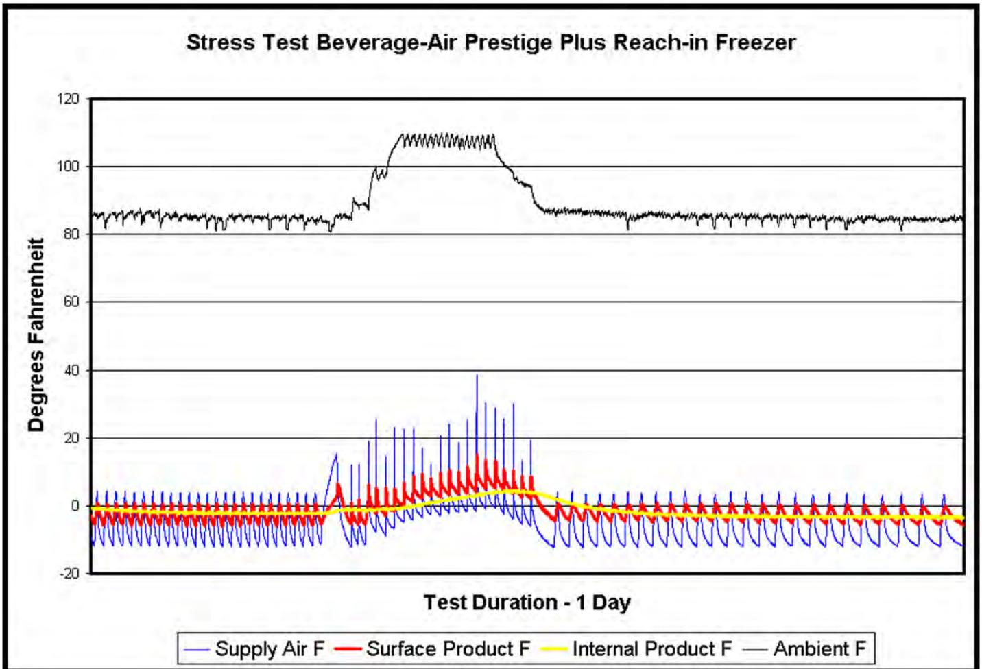
Between five and six hours, the change was dramatic until the temperature warmed due to a frosted coil and the inability to properly circulate air. After 10 hours the freezer was unable to cycle and steadily lost temperature.
